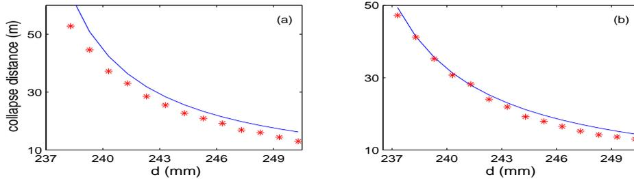
Fig. 1 Experimental (stars) and theoretical (solid line) results of the collapse distance as a function of  $d$  for powers of (a) 2 TW and (b) 3 TW.
