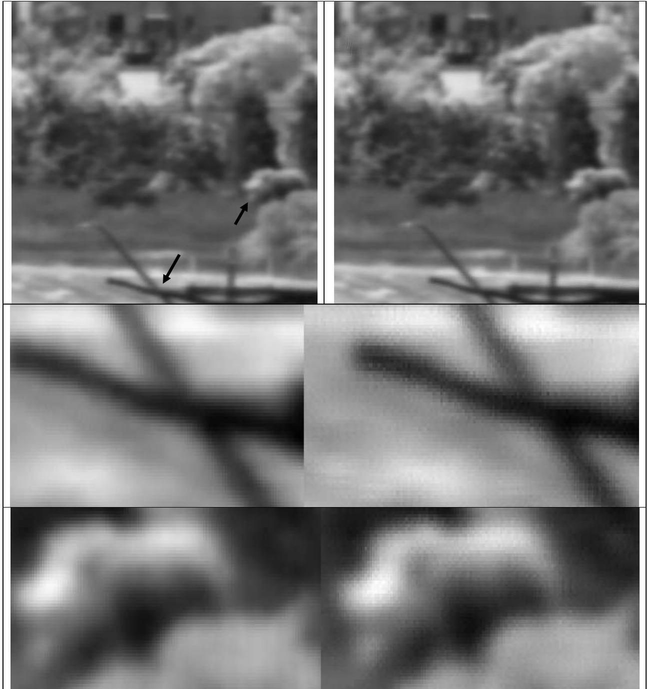
*Super Resolution from Turbulent Motion. The left-hand side is the stabilized image extracted from a real life sequence. The right-hand frame is the same frame with super-resolution applied.*
