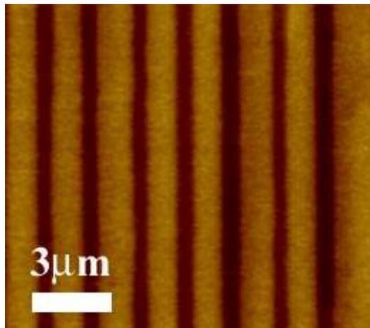
Piezoresponse force microscopy images of nanodomain grating fabricated in stoichiometric LiTaO<sub>3</sub> sample under low relative humidity.
