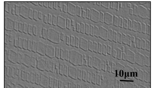
Figure 2: Microscope picture of the +Z side of the etched structure. The parallelograms are the inverted domains with sides of  $3.6\mu\text{m}$  over  $12\mu\text{m}$ .
