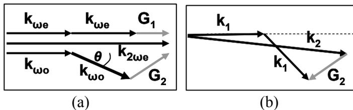
Figure 1: QPM vector schemes of (a) an all-optical deflector based on two cascaded interactions of SHG and DFG and of (b) the SFG experiment to characterize the 2D PPSLT.
