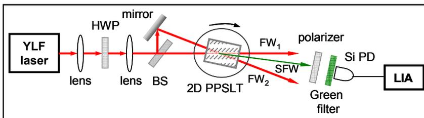
Figure 3: Experimental setup for characterizing the 2D PPSLT.
