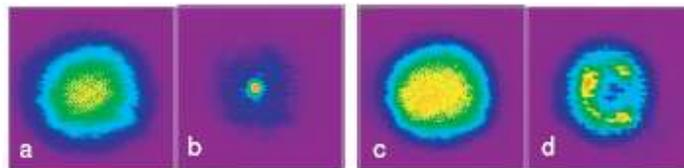
Figure 1. Images of the input and output intensity beam profiles for a 7-cm propagation distance (0.9 mm X 0.9 mm). (a) Gaussian input profile, (b) output beam with the Gaussian input and an input energy of  $E = 5.6 \mu\text{J}$ , (c) super-Gaussian input profile, (d) output beam with a super-Gaussian input and an input energy of  $E = 5.0 \mu\text{J}$ .
